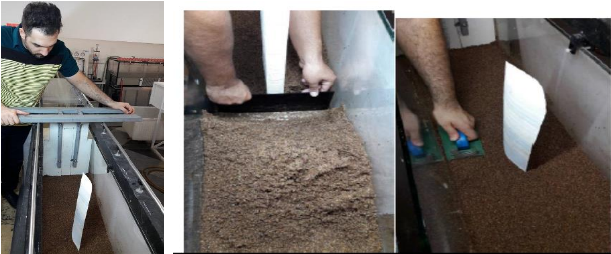
Figure 3: levelling the deposits located around the pier
