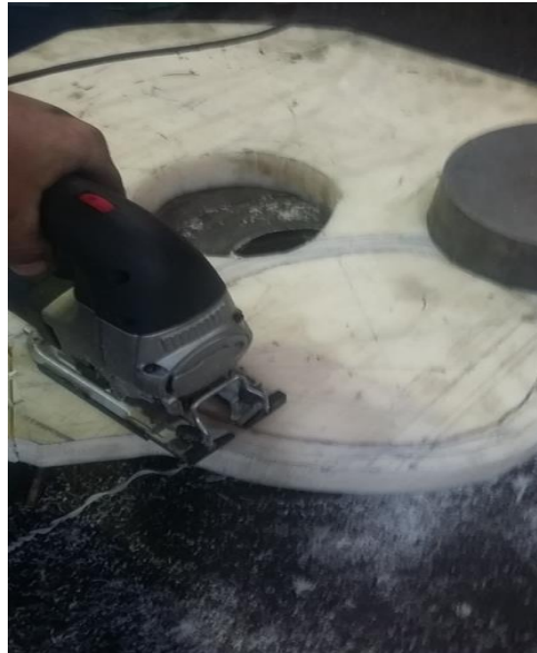
Figure 2- cutting the design by chain saw upright on white Teflon
